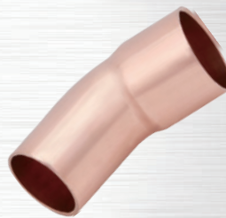
T202 45° Elbow with Single Socket (C × Ftg)
